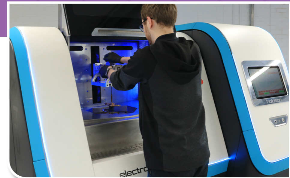
Henry Bramwell operating Holdson's electroform machine, which is up to six times faster than other post-processing methods and systems.
