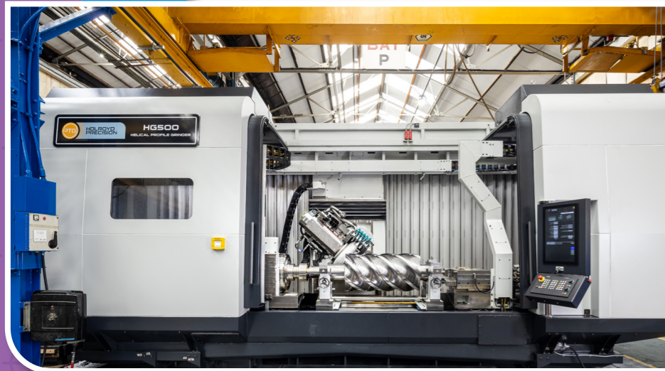
510mm diameter compressor rotor inside the PTG Holroyd HG500 helical grinding machine.
